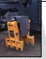
Coming Soon! Hydraulic powered dual tamper head with innovative approach using little or no track time
