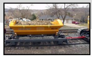
**Side Dump Cart**—Features 180 degree rotation to easily handle all types of materials from the comfort of the cab
