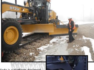
The Rail Blade is a platform designed for versatility. The new **Tie Inserter/ Remover** attachment makes it easy to maintain and repair switch ties.
