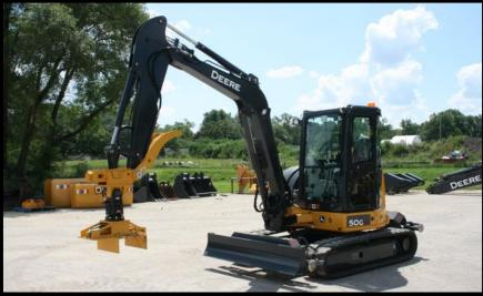
Meet the new 50G Bridge Excavator! This modified compact excavator was designed specifically for bridge work, featuring ramp clamps to hydraulically clamp to the rail for increased stability and safety. The excavator arm (instead of tie boom) provides extra maneuverability. An optional tie head that clamps and slides is also available.
